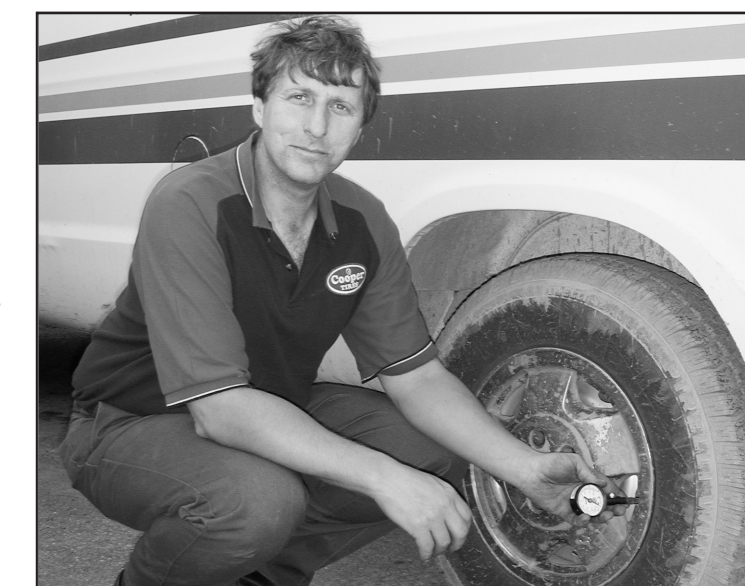
Marc Pinkus, owner and manager of Pinkus Tire and Battery in Williamsburg, demonstrates how to measure tire pressure with a gauge. He recommends tire pressure should be measured on a regular basis.
