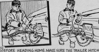
IS SECURELY FASTENED AND SAFETY CHAINS ATTACHED. CHECK TRAILER LIGHT CONNECTION, AND TEST TO SEE THAT LIGHTS WORK PROPERLY. AR
