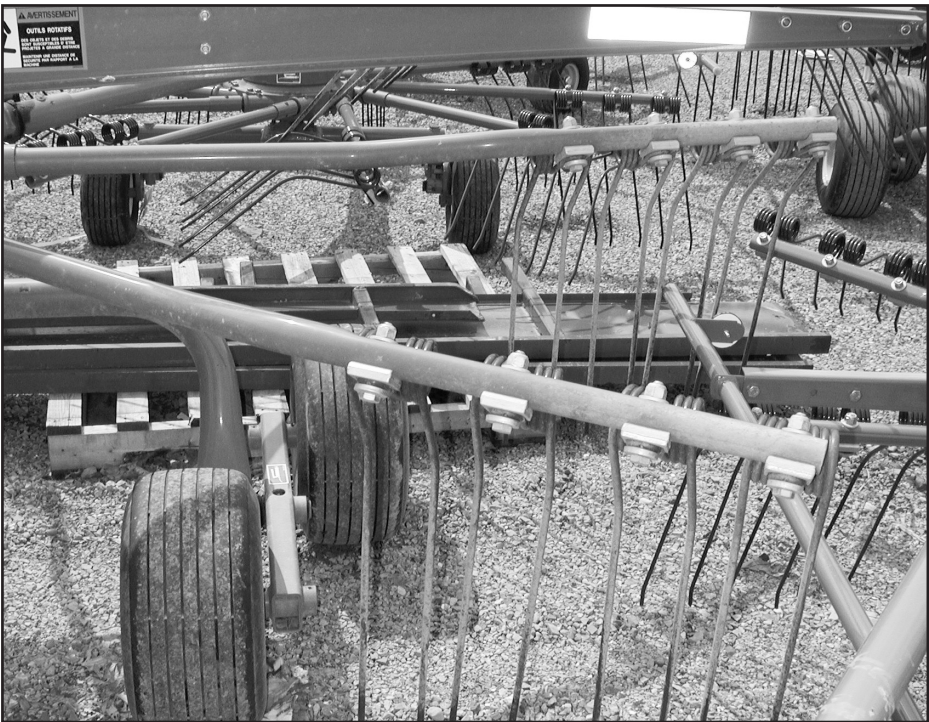
The double-bent tangential tine arms of the Kuhn Gyorake and the high bend of its teeth, allow for a smooth and straight motion, minus the unwanted debris.
