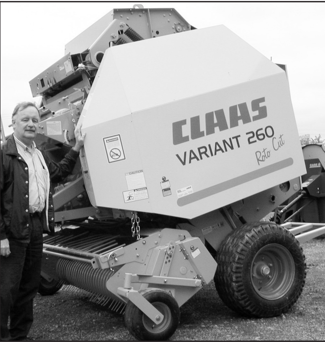
The Claas Variant 260 allows forage harvesters to choose how large they want their round bales to be, from 36 inches to 60 inches in diameter. The baler also can be adjusted to produce different bale densities, to adapt to field conditions during harvest. Hugh Hodgins is the general sales manager at Reis Equipment Centre in Winchester which has sold Claas products for the past 10 years. Press Photos — Zabel
